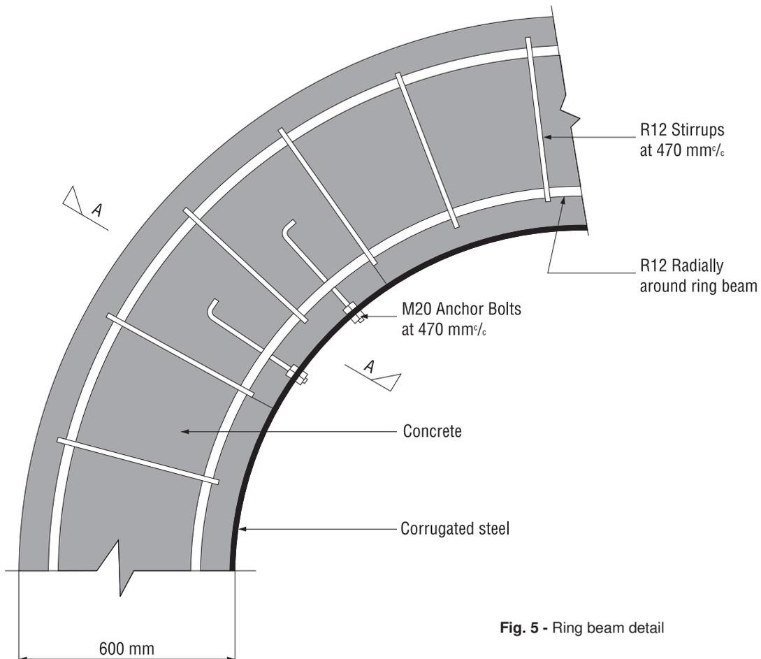
Fig. 5 - Ring beam detail
