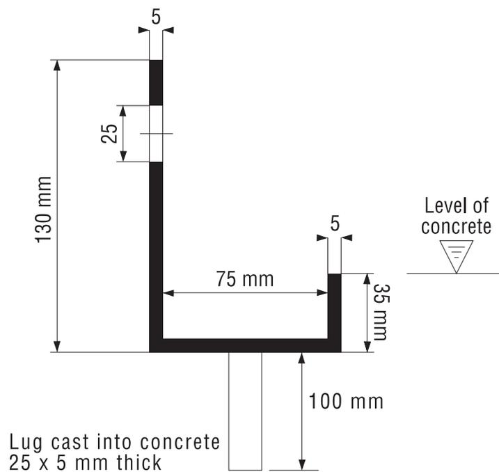
Fig. 6 - Unbalanced channel for MP200 Arches
