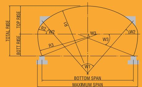
**Super-Span Low Profile Arch SSLA**
