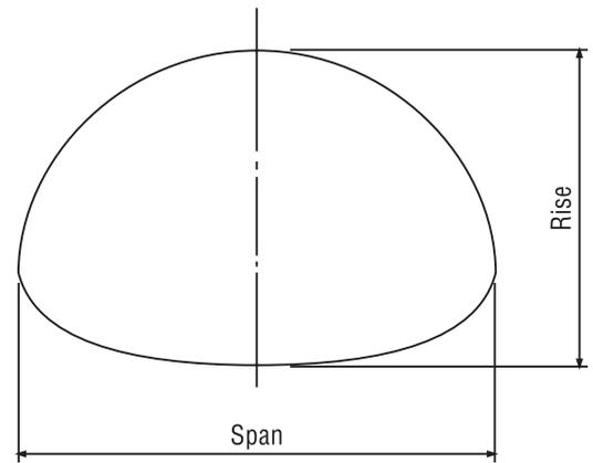
**Fig. 5 - NPA Pipe Arch**
